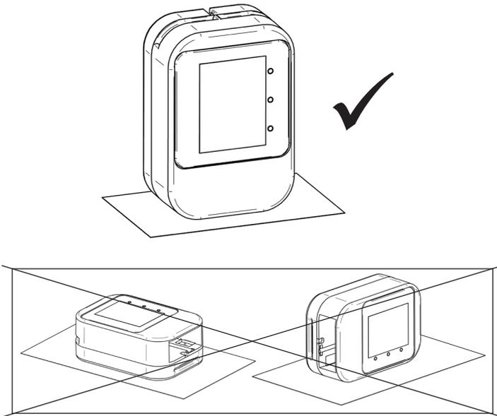
3. Once the Condair Cube is in place, it requires an adjustment time of approx. 20 minutes until all values are displayed correctly. In particular, the temperature may deviate during the first phase after switching on, since the sensor is not yet at operating temperature.
