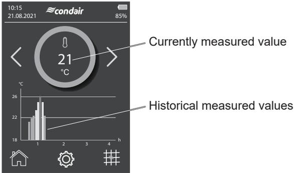
This view shows the course of the measured room temperature over a maximum of 4 hours.
