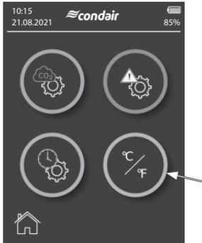
2. Switch between degrees Celsius / degrees Fahrenheit by pressing the icon. The set value is displayed in the lower gray box with °C or °F.
